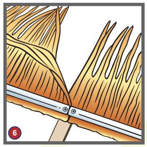
6) At a rail junction, you must create an overlap of a minimum of 5 cm (2") between the leaves on the new rail to the leaves already installed on the first rail.
